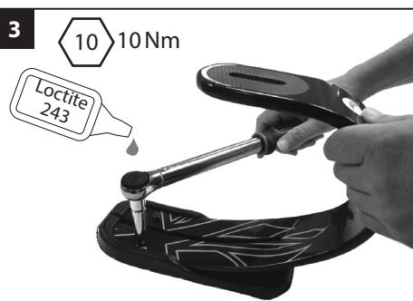
Fit the Toe Spring into the Heel spring cover and tighten the bolts to 10 Nm.
