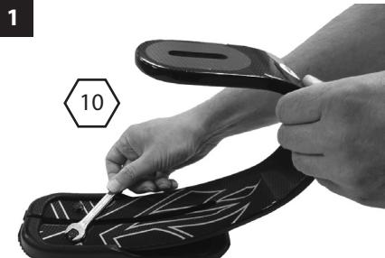
Undo the 2 Heel Spring retaining bolts.
