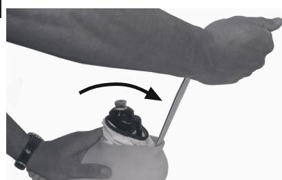
Rotate shoe horn as shown to remove shell.
