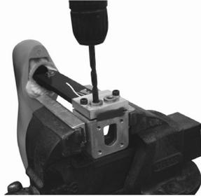
Drill two 8.1mm diameter holes through drill bushes.
