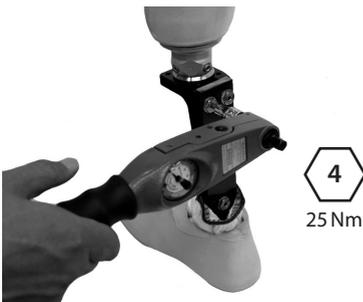
Loctite (243) & tighten (25 Nm) top housing bolts. Attach and align socket.
