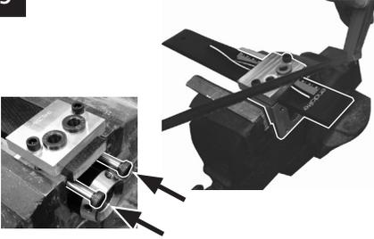
Remove socket, place fitting clamp in the vice and cut blade to length. Fit shoulder screws to prevent damage to components
