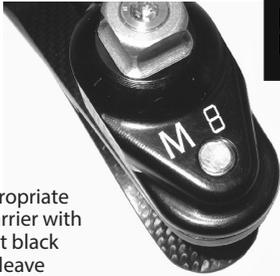
Cover appropriate lines on carrier with permanent black marker to leave spring set number showing.
