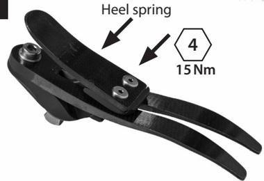
Assemble heel spring onto carrier, use Loctite 243 (926012) and torque to 15 Nm.
