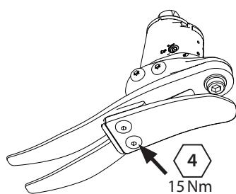
Re-assemble with replacement heel spring. Use Loctite 243 (926012) and torque to 15 Nm.
