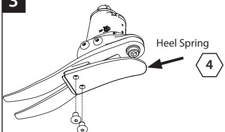
Remove heel spring and screws.
