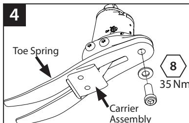
Remove toe spring screw, replace toe. Upon reassembly, use Loctite 243 (926012) and torque to 35 Nm. Ensure toe spring is central to the carrier.
