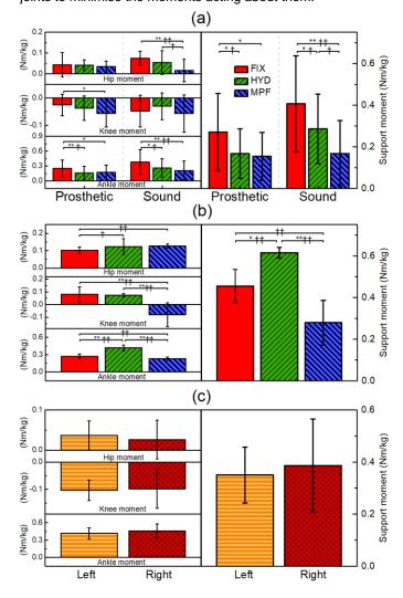
**Figure 2:** The relative contributions of ankle, knee and hip moment to the total support moment for (a) unilateral trans-tibial amputees, (b) a bilateral trans-tibial amputee and (c) able-bodied control participants. Asterisks indicate statistical significance: p<0.05, \*p<0.01. Obelisks indicate effect size changes: t|d|>0.5, tt|d|>0.8.
