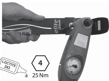
Attach pylon to heel carrier. Loctite (243) & tighten bolt (25 Nm).
