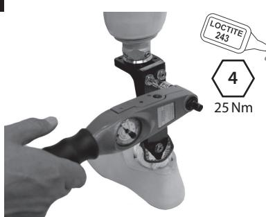
Cut pylon using method shown previously before attaching top housing. Loctite (243) & tighten bolts (25 Nm). Re-apply cosmesis if applicable.
