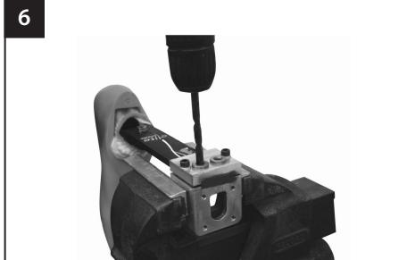
Drill two 8.1 mm diameter holes through drill bushes.
