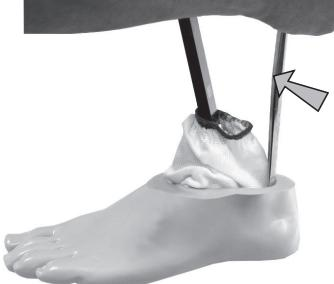
Using a lever, ease assembly into shell.
